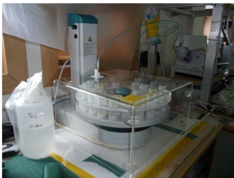
Figure 19. The voltammetric equipment with in front the sample changer. The electrode stand is mounted in a NIOZ home-made aluminium frame on a wooden board that is hanging in elastic bands, preventing scans to be disturbed by motions of the ship. At the left is a sample that was taken to test the influence of bacterial activity on the characteristics of the ligands. The sample is kept in the laboratory at room temperature to stimulate bacterial activity.
