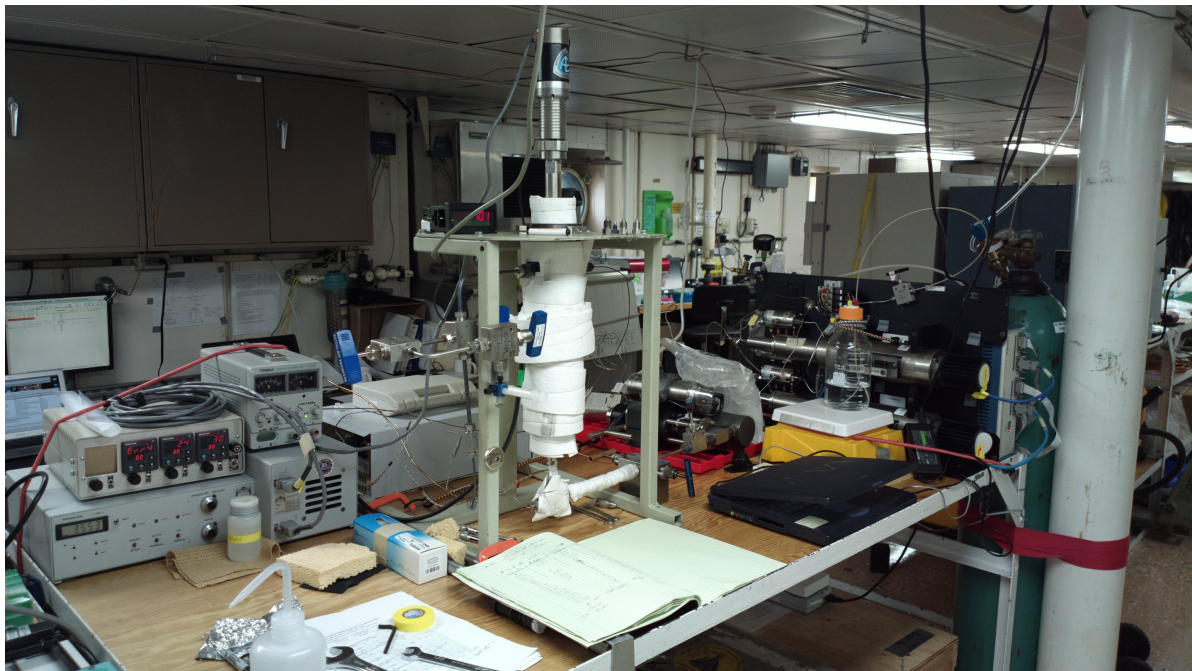
Figure 2. The CIW high-pressure bioreactor deployed onboard the R/V Atlantis. Continuous culturing experiments of microbial communities from Crab Spa and Tica were conducted at in-situ pressure (250 bar) and temperature (30-50°C) conditions by integrating vent fluid sampling techniques (Isobaric-Gas-Tight sampler, WHOI) with our experimental facility.
