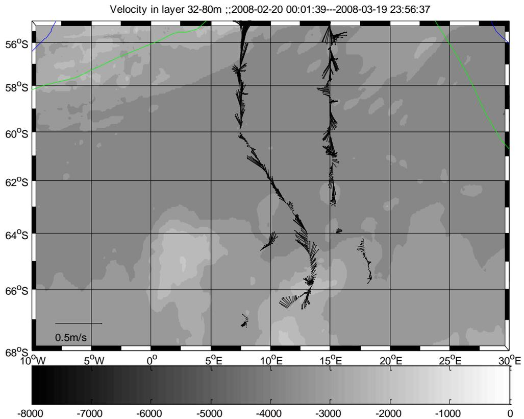
Figure 3.11 The horizontal currents in the southern region from the shipboard ADCP-75kHz.
