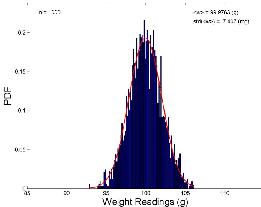
Figure 13.4. The PDF and a Gaussian PDF fit (red) of 1000 weight measurements of an 100-g standard weight. There are 5 runs with each including 1000 weighing values. The mean and the standard deviation of the 5 runs are given in the legend.
