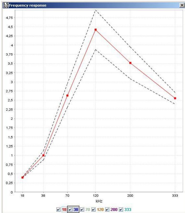
Figure 8.1. Frequency response of krill.
