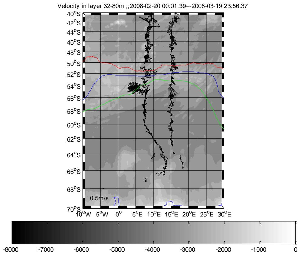
Figure 3.9 Large-scale overview of horizontal currents from the shipboard ADCP- 75kHz.
