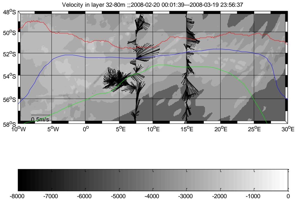
Figure 3.10 Blow up of the horizontal currents in the main frontal region from the shipboard ADCP-75kHz.
