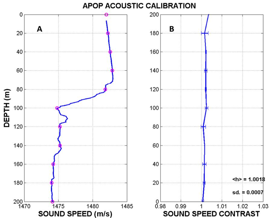
Figure 13.3. A) The water column sound speed based on temperature and salinity and B) the APOP sound speed contrast calibration profile conducted on 17 March 2008.
