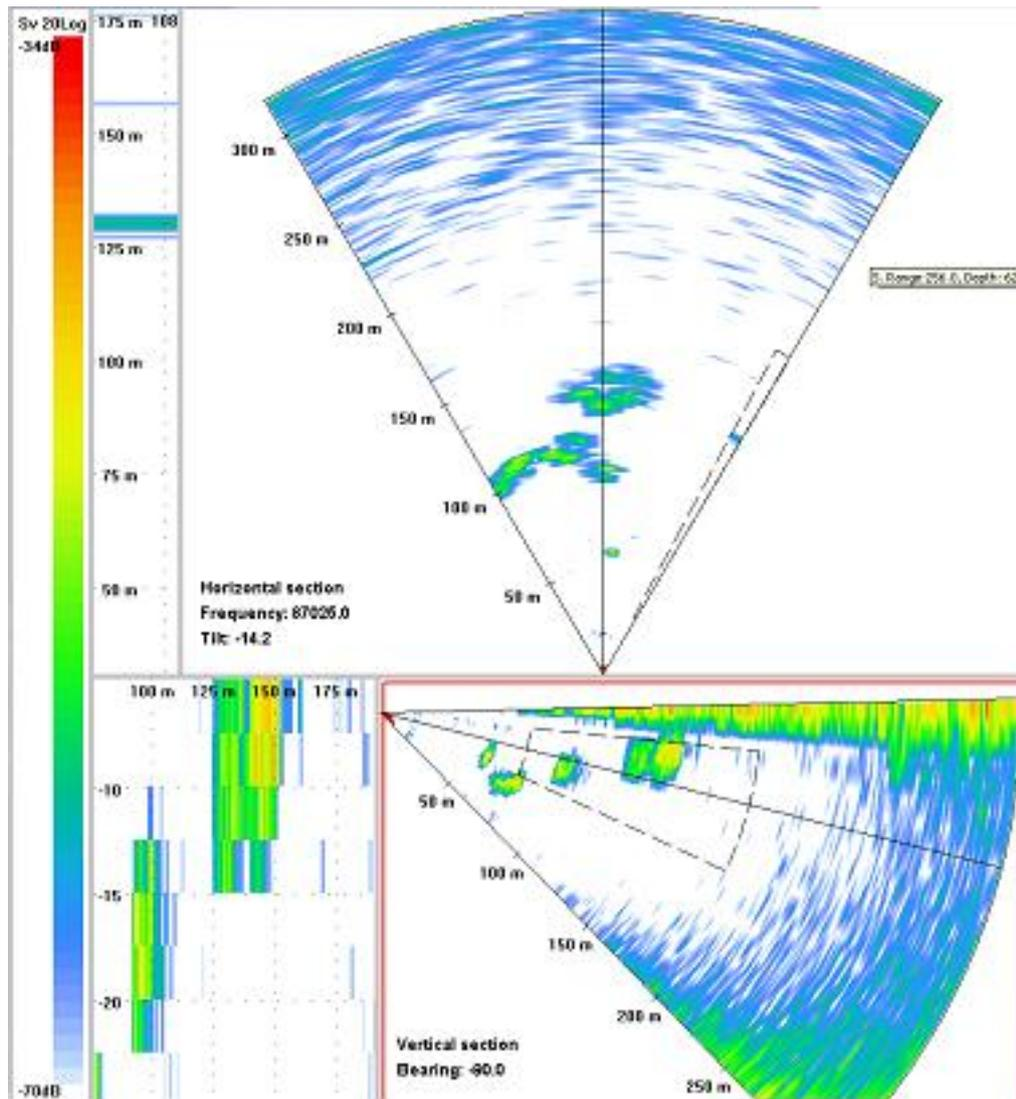
Figure 10.1. Sonar screendump 29.02.08 (64°31 S, 017°50 E) produced from Simrad MS 70 multibeam sonar. The picture is showing krill schools of various dimensions and densities within 150 m from the port side of the vessel and distributed shallower than 22 m depth.
