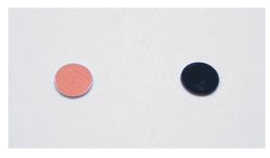
Fig. 7 Sensor spot back (red) and front (black)
