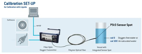
Fig. 12 Calibration set-up: Two-point calibration of a PSt3 sensor spot with liquid calibration standards
