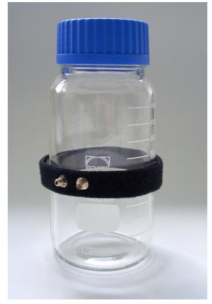
Fig. 4 Adapter for round containers (ARC)
