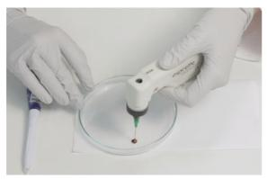
Fig. 10 Carefully place the oxygen sensor spot in the vessel
