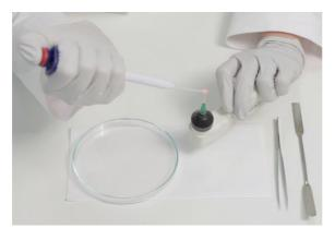
Fig. 9 Applying silicon glue to the sensor spot
