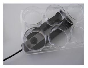
Fig. 5 Coaster CFG used to read the response of an oxygen sensor spot in a 6-well multidish
