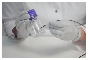
**Fig. 11** Polymer optical fiber held by hand opposite the sensor spot to read its response
