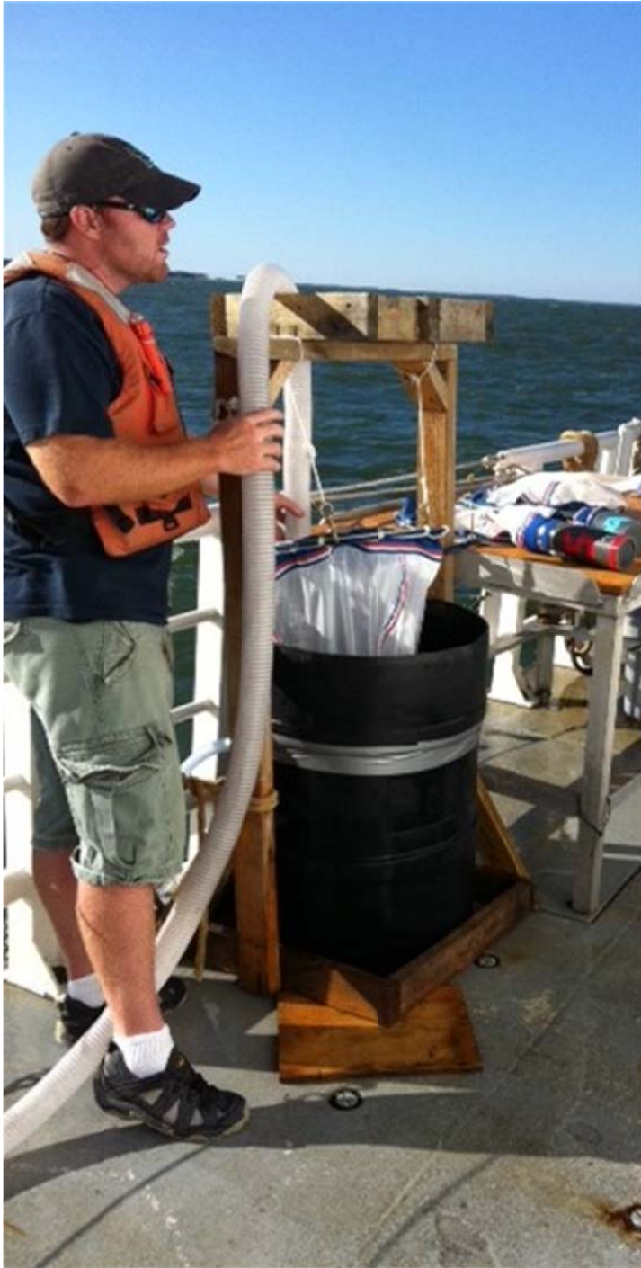
Fig. 2. Jake Goodwin directing hose into plankton net which was suspended inside a 50 gallon drum filled with water ( \frac{3}{4} full) to ensure the plankton were cushioned and not forced through the mesh by the high-volume pump. A series of small holes above the duct tape allowed water to drain out and maintain the drum \frac{3}{4} full.
